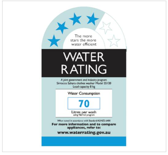
The WELS label shows water use efficiency and total water consumption for the appliance.
