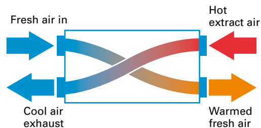
Figure 14 Principle of operation of a recuperator
