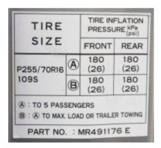
You can improve your gas mileage by up to 3.3% by keeping your tires inflated to the proper pressure. Under-inflated tires can lower gas mileage by 0.3% for every 1 psi drop in pressure of all four tires. Properly inflated tires are safer and last longer.<sup>1</sup>
