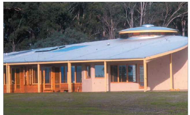
Covered balconies should allow winter sun access.
